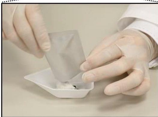
Sorbent for dehydrating samples with high water content
